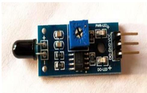
It is used to identify infrared signals and generate electronic pulses and transmit them to processors
