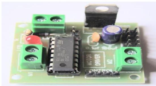
It controls speed and direction of two motors simultaneously
