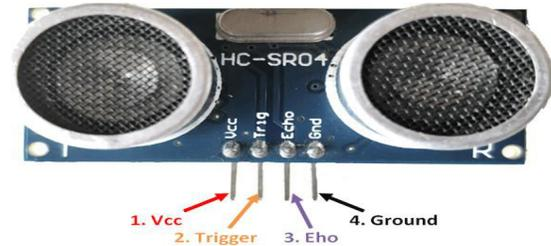
It is used to detect the objects present in front of it by ultrasonic waves.
